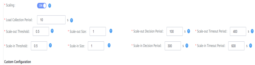
Figure 8-2 Scaling out/in an instance
